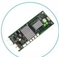
Tke display board MS3-E V2.0/MS5-E2.1
