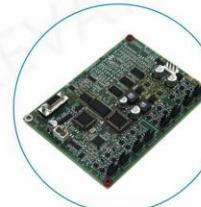
Otis load weighing board GBA26800KJ1
