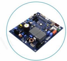
Door machine board CTC REV 2.0
