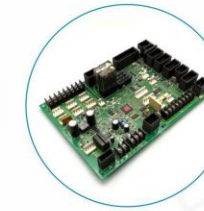
Fujitec door machine board IF66A F/J
