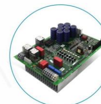
Otis inverter drive board GAA26800KN1
