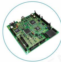
Toshiba main board PU-100A/UCE1-322C13
