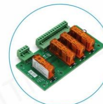
Relay board MCTC-SCB-D/A
